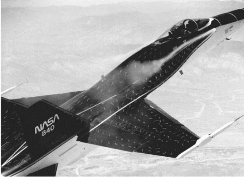
Figure 1. Flow visualization of the F-18 HARV vortex breakdown ahead of the vertical tails. Photograph courtesy of the NASA Dryden Flight Research Center.
